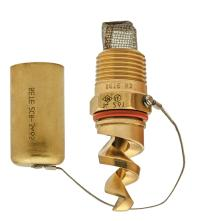
**Fan and Deflected Fan Nozzles**: Fan nozzles are used in water wall fire protection systems because they provide an adequate barrier to shield personnel and equipment against radiant heat, harmful gases, and flames. These nozzles are designed for effective spray impact, and deflected fan nozzles produce an extra-wide spray pattern allowing more water to spray and form a suppression wall.
