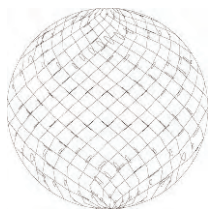
Orbitor 2 nozzle spray pattern
