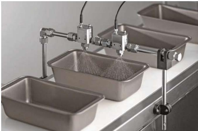
The spray flow rate can also be electronically controlled by pulsing the sprays while adjusting the ratio of ON versus OFF dwell time within each cycle. Pulsing at high frequency allows the average flow rate to be adjusted while maintaining constant fluid supply pressure and the appearance of continuous, uniform coverage. This flow control process is known as Pulse Width Modulation (PWM).
